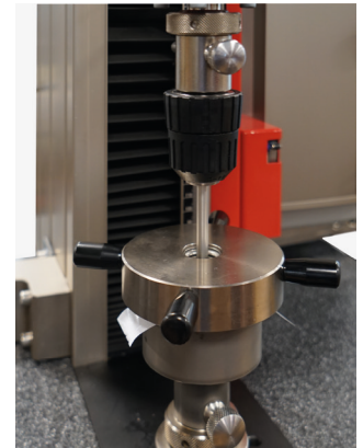
Puncture test on separator film
