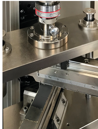
Z-direction tensile test on electrode coating
